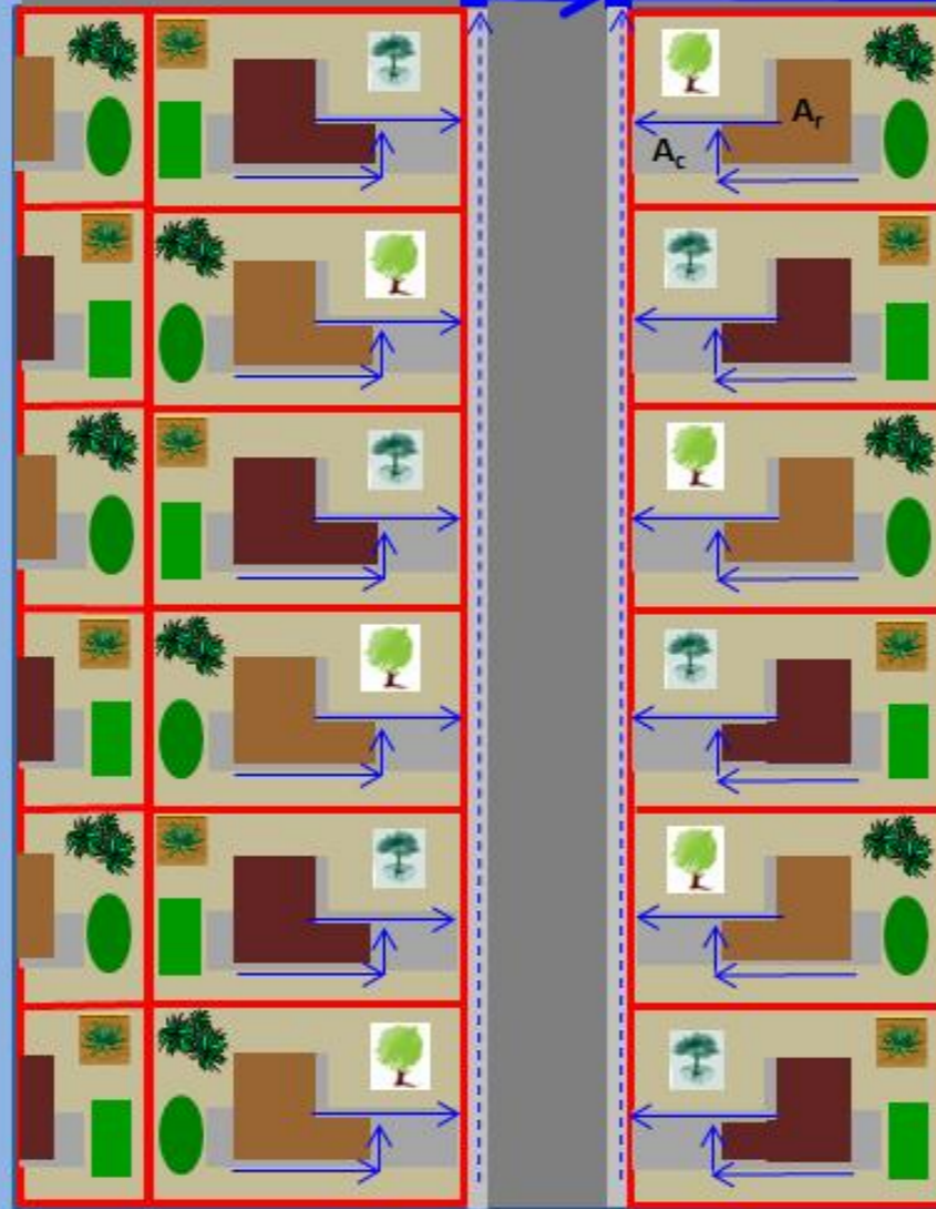
Existing Subdivision With Paved Streets, Concrete Gutters and Storm Drainage Collection Facilities
